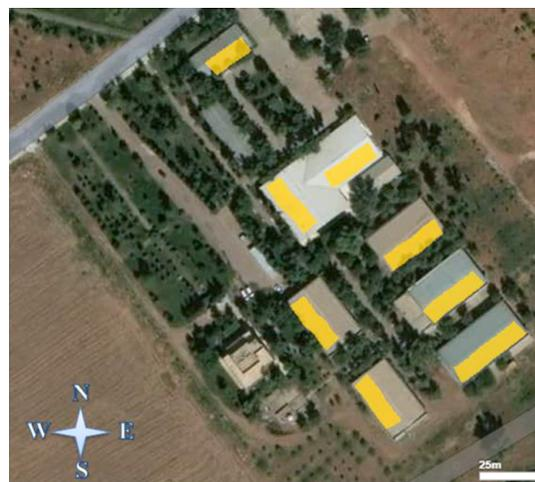
**Figure 1. Roof surfaces of Vocational School of Technical Sciences that can be used for the electricity generation by PV system**
