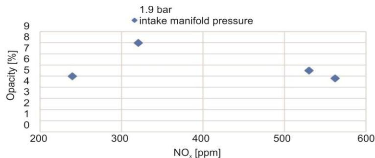
**Figure 9. The NO<sub>x</sub>/soot trade-off of the TPO for the third operating case, listed in tab. 2**
