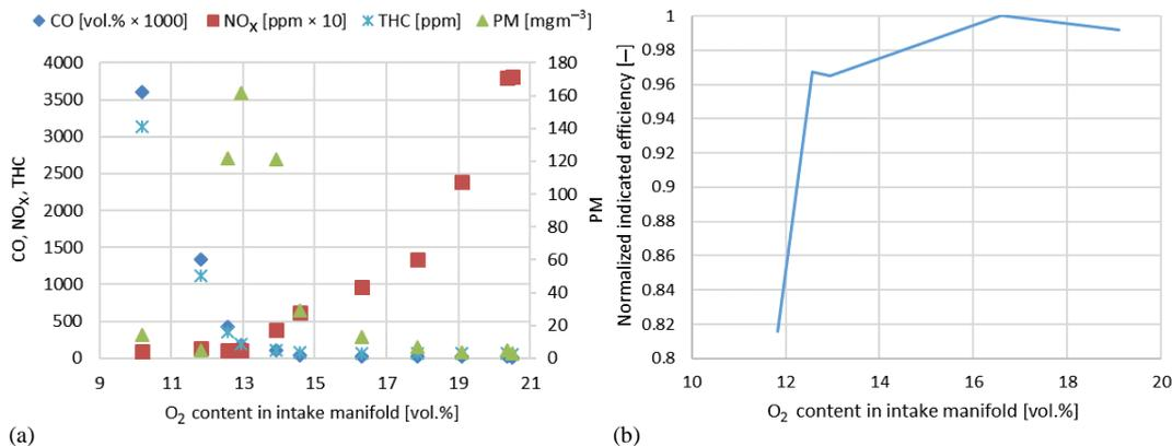
Figure 4. Exhaust gaseous emissions with PM (a) and normalized indicated efficiency of the D2 for the first operating mode (b), listed in tab. 2
