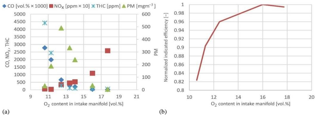
**Figure 7. Exhaust gaseous emissions with PM (a) and normalized indicated efficiency of the D2 for the second operating mode (b), listed in tab. 2**
