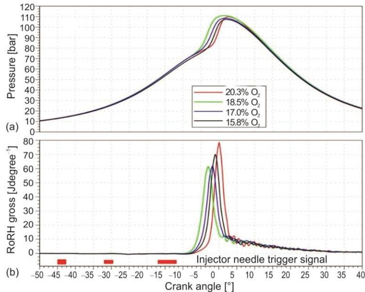
**Figure 8. Pressure traces (a) and ROHR of the TPO for the third operating mode (b), listed in tab. 2 (for color image see journal web site)**
