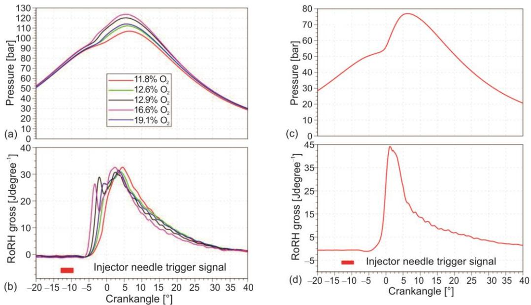
**Figure 2.** Pressure traces (a), (c) and ROHR (b), (d) of the D2 for the first operating mode, listed in tab. 2 with higher – 2.25 bar (a), (b) and lower – 1.19 bar (c) and  $p_{IM}$  (d) (for color image see journal web site)
