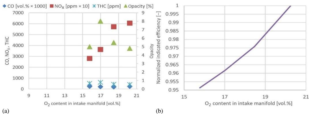
**Figure 10. Exhaust gaseous emissions with opacity (a) and normalized indicated efficiency of the TPO for the third operating mode (b), listed in tab. 2**
