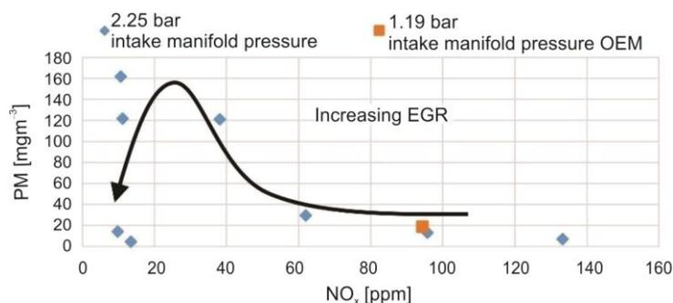
**Figure 3.** The  $NO_x$ /PM trade-off of the D2 for the first operating mode, listed in tab. 2
