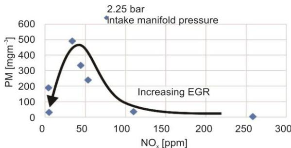
**Figure 6.** The  $\text{NO}_x$ /PM trade-off of the D2 for the second operating mode, listed in tab. 2
