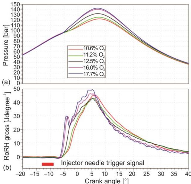
**Figure 5.** Pressure traces (a) and ROHR of the D2 for the second operating mode (b), listed in tab. 2 (for color image see journal web site)
