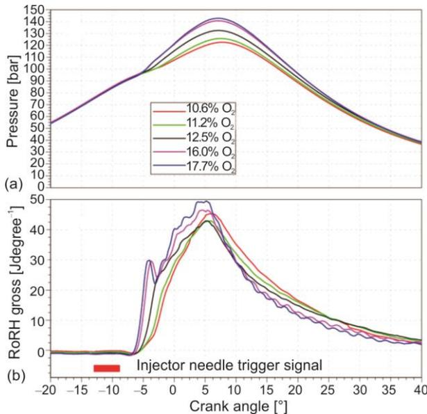
**Figure 5. Pressure traces (a) and ROHR of the D2 for the second operating mode (b), listed in tab. 2**
