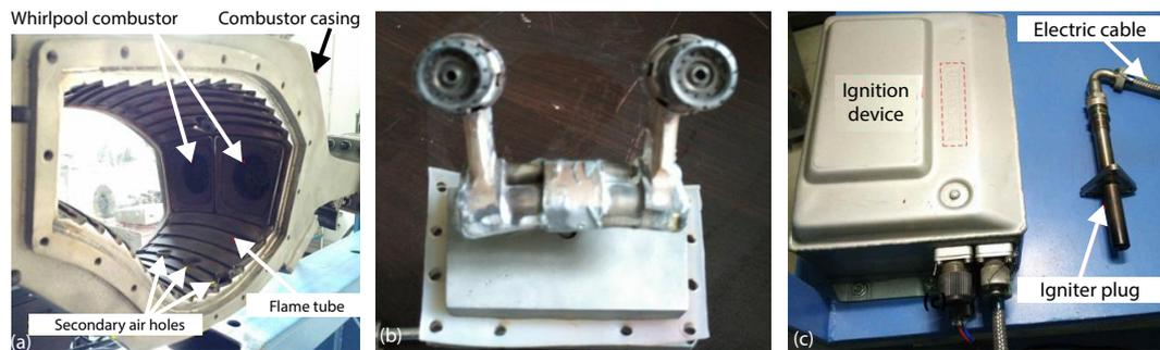
Figure 2. Components of PAC test facility; (a) flame tube and annular combustor casing, (b) fuel spray nozzle, and (c) ignition equipment
