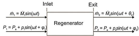
Figure 2. Regenerator schematic with important modeling parameters
