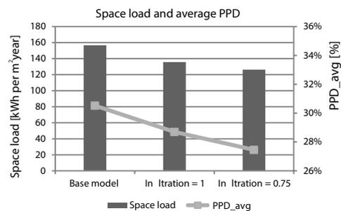
Figure 10. Yearly space conditioning load and the average PPD for different infiltration rates
