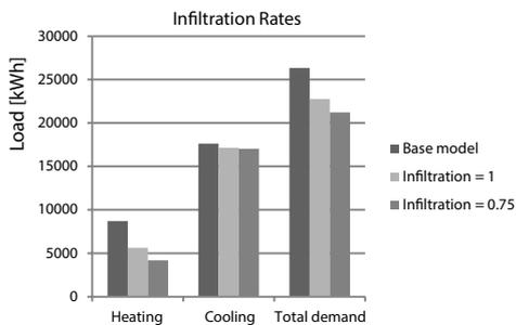
Figure 9. Simulation results for different infiltration rates
