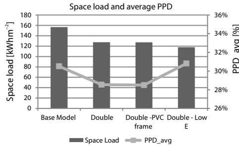
Figure 8. Yearly space conditioning load and the average PPD for different glazing design alternatives
