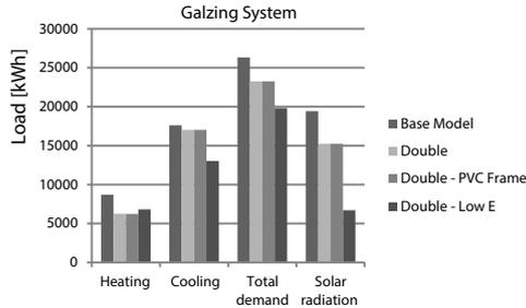
Figure 7. Simulation results for different glazing design alternatives
