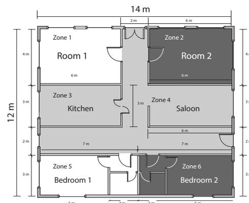
Figure 2. Thermal zones for the house model
