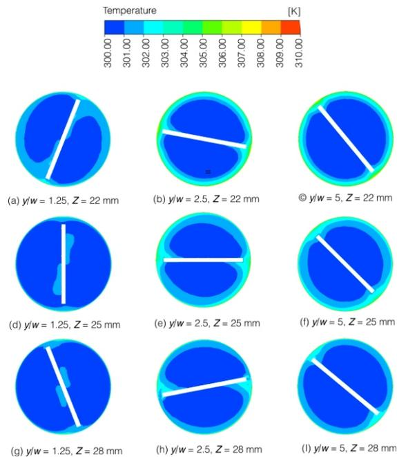
**Figure 5. Temperature distribution with respect to various twist ratios**
