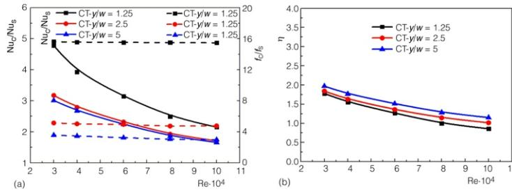
**Figure 3. Effect of the twist ratio on flow and heat transfer performance**
