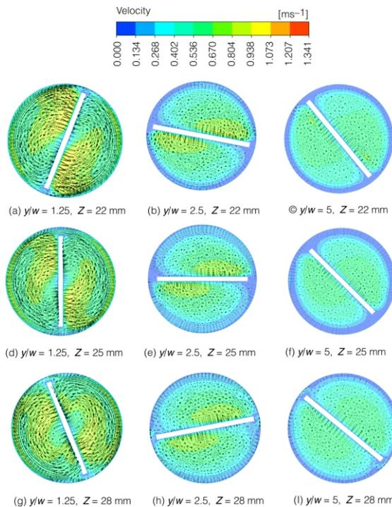
**Figure 4. Velocity vector distribution with respect to various twist ratios**
