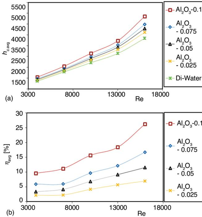
Figure 4. (a) Average heat transfer coefficient of Di-water and Al<sub>2</sub>O<sub>3</sub>-water nanofluids over a BFS and (b) average heat transfer coefficient enhancement vs. Reynolds number
