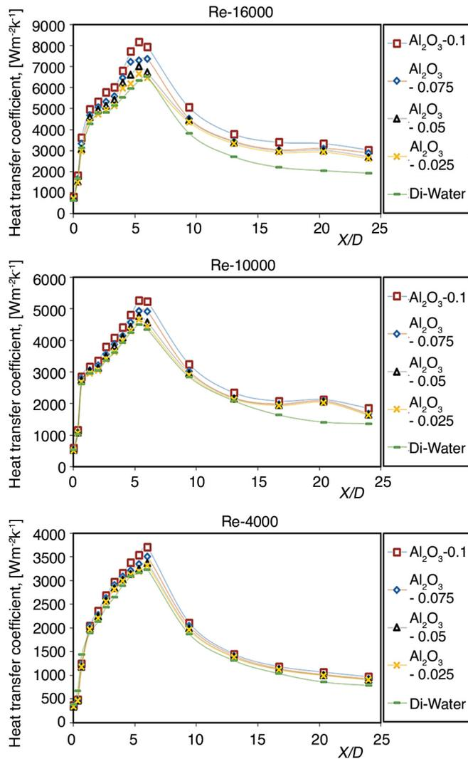
**Figure 5.** The effect of Reynolds numbers and weight concentrations of Al<sub>2</sub>O<sub>3</sub>-water nanofluids on the local heat transfer coefficient at different axial ratios
