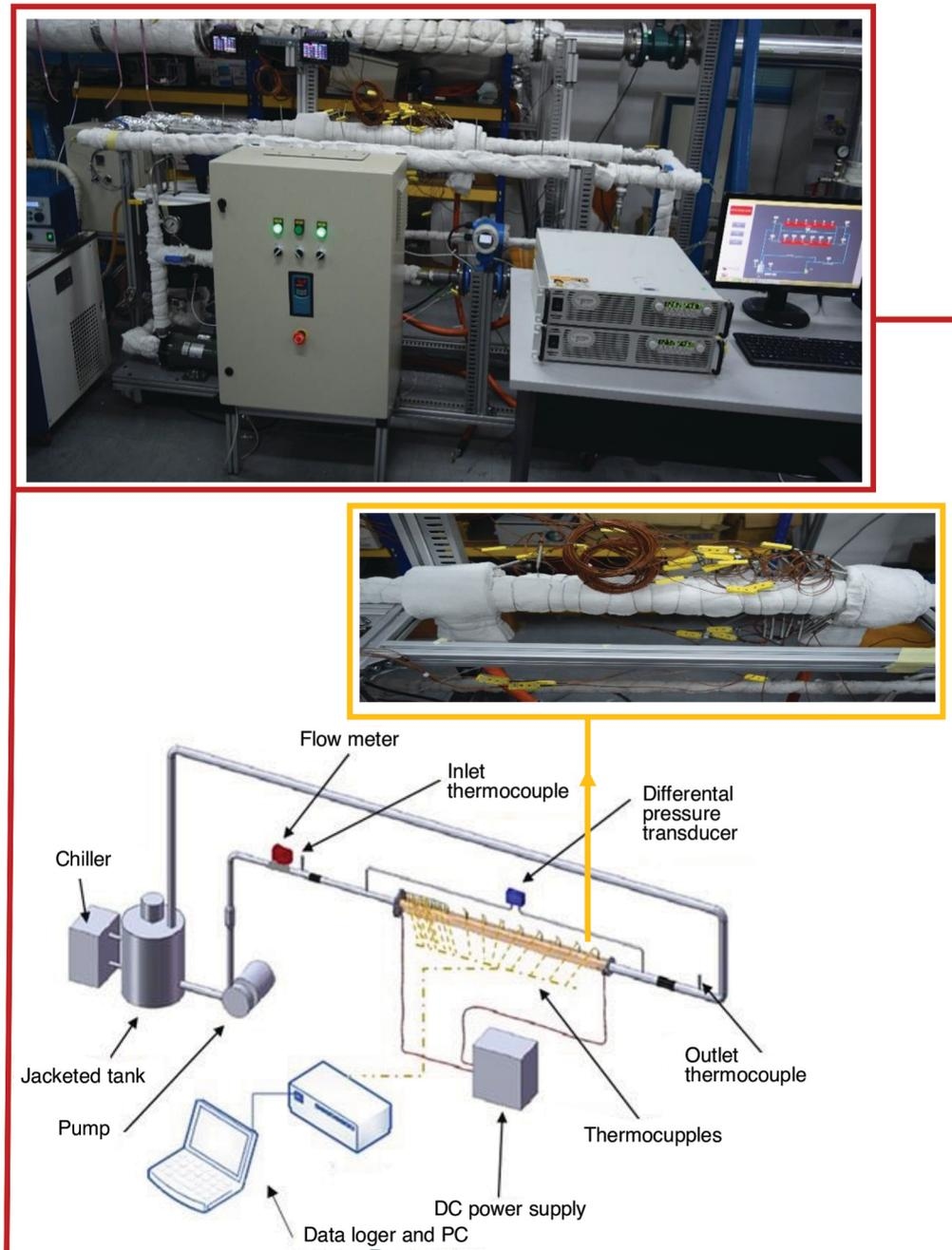
Figure 1. Schematic diagram of the experimental set-up
