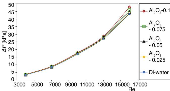
Figure 7. Experimental pressure drop of Di-water and Al<sub>2</sub>O<sub>3</sub>-water nanofluids at weight concentrations of 0.025 wt.%, 0.05 wt.%, 0.075 wt.%, and 0.1 wt.%, for different Reynolds number.
