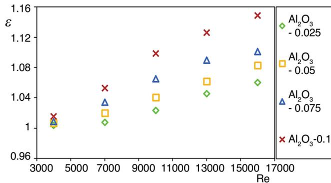
Figure 6. Performance index for the BFC in the presence of Di-water and Al<sub>2</sub>O<sub>3</sub>-water nanofluids with different weight concentration.
