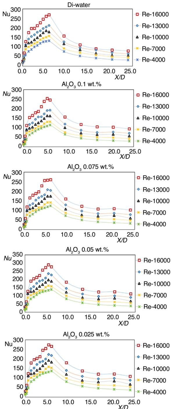
Figure 3. Experimental Nusselt number of Di-water and  $Al_2O_3$ -water nanofluids at different weight concentrations of 0.025 wt.%, 0.05 wt.%, 0.075 wt.%, and 0.1 wt.% for different Reynolds numbers.
