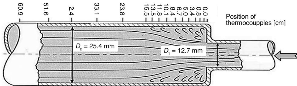
Figure 2. Schematic view of the test section
