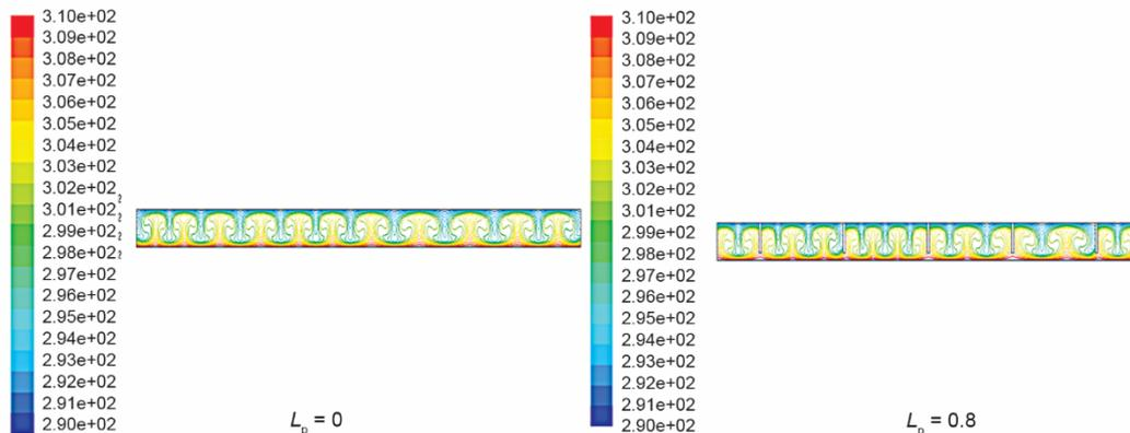
**Figure 5. Isotherms for different values of  $L_p$  for  $Ra = 2.51 \cdot 10^4$ ,  $N = 5$**
