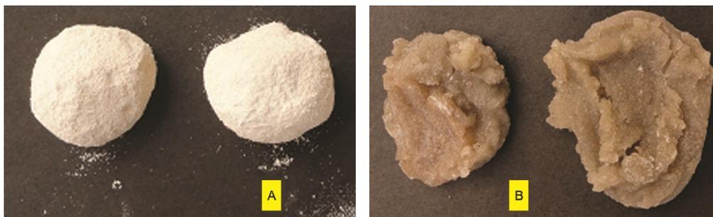
Figure 1. Pellets of catalyst; (A)  $\text{CeO}_2$ , (B)  $\text{SiO}_2$
