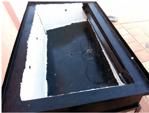
Figure 4. Pictorial view of modified solar still with cotton cloth
