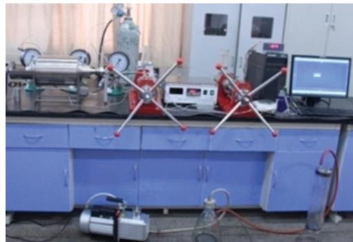
Figure 2. Triaxial gas seepage testing system
