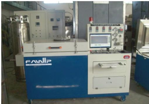
Figure 1. The SLX-80 high and low temperature treatment system
