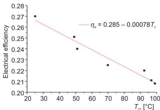
Figure 5. The electrical efficiency varies with  $T_c$
