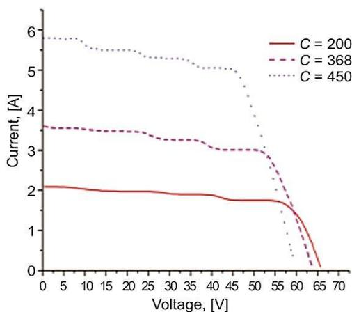
Figure 6. The I-V curves of the PV module under different concentration ratio
