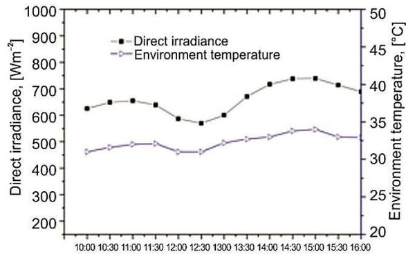
Figure 4. Direct irradiance and environment temperature vary with local time
