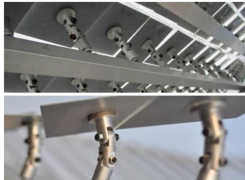
Figure 2. The photograph of universal joint using in plane mirror system
