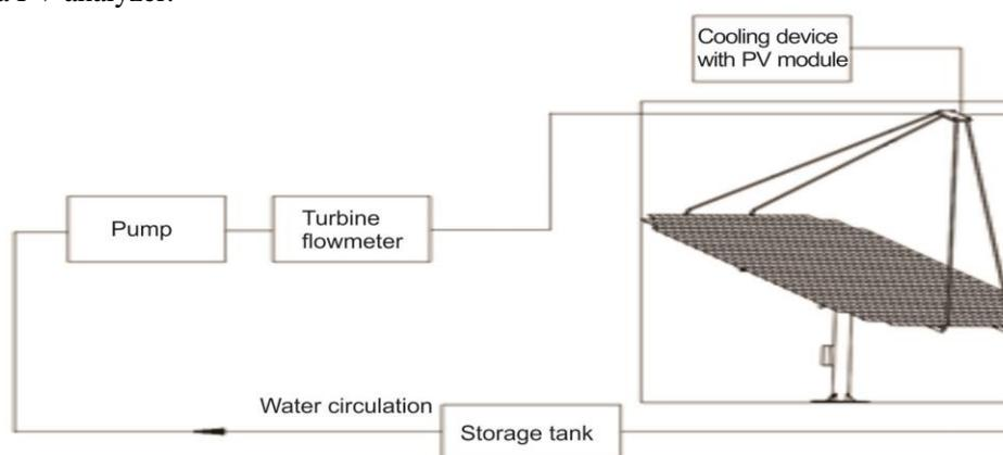
**Figure 3. The experimental test system of the HCPV/T system**
