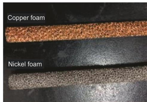
**Figure 2. Copper and nickel foam**
