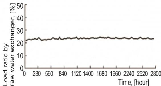
Figure 10. Load ratio by raw water exchange in SCW
