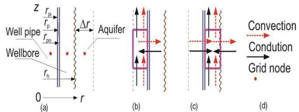
**Figure 2. Sketch maps of the heat transfer in the drawing pipe, well hole, and well pipe; (a) size sample, (b) well pipe, (c) wellbore, (d) legend**
