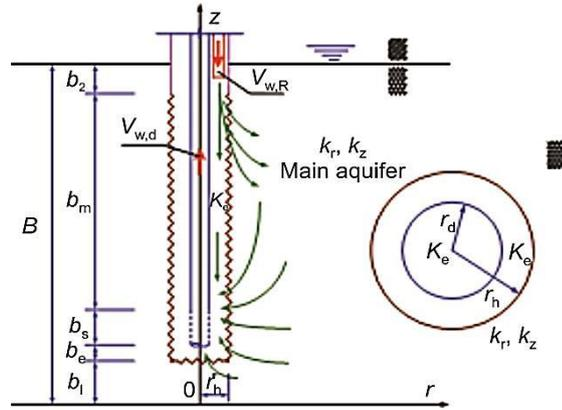
**Figure. 1 Schematic diagram of the water flow model**
