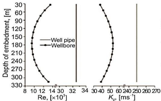
**Figure 7. Reynolds number and vertical EHC in drawing pipe and well hole**
