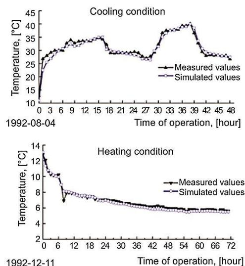
**Figure 3. Comparison of drawing water temperature between the simulation and experiment**
