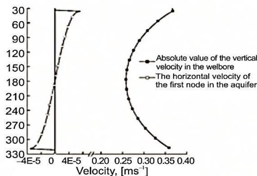
Figure 6. Velocity in the well hole and aquifer vs. depth
