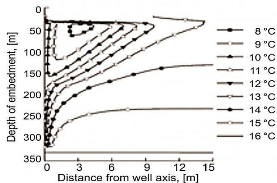
**Figure 9. Temperature contour of the aquifer at the end of heating season**
