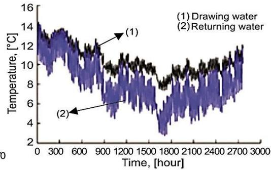
**Figure 8. Drawing and returning water temperature of SCW vs. time**
