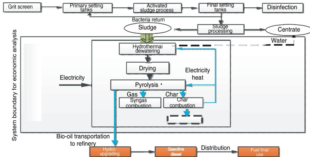
Figure 1. Process schematic for sludge pyrolysis system and boundary for economic analysis
