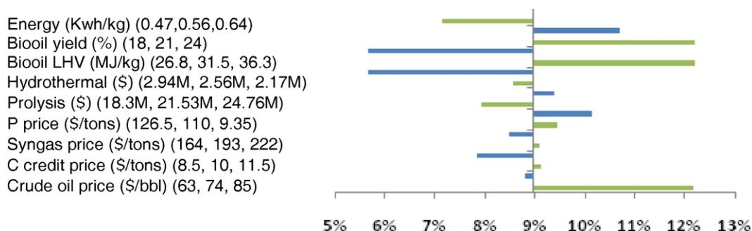
Figure 3. The SA of sludge pyrolysis production system
