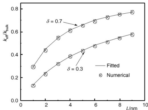
**Figure 5. Fitted result of effective thermal conductivities of SiO<sub>2</sub> nanograin at 300 K**
