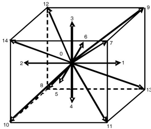
Figure 2. The D3Q15 model
