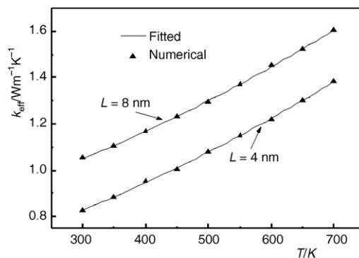
**Figure 6. Fitted result of effective thermal conductivity of SiO<sub>2</sub> nanograin at different temperatures**
