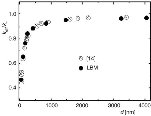
Figure 3. Comparison of normal thermal conductivity in Si films at 300 K
