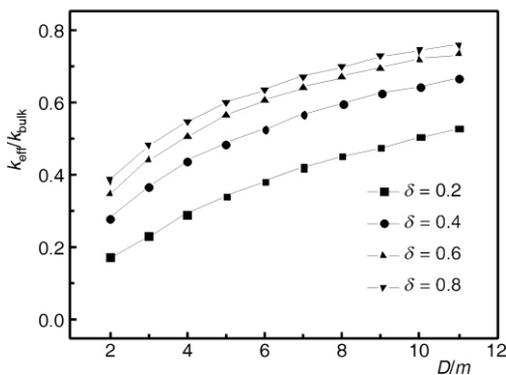
Figure 4. Effective thermal conductivities changing with the nanograin diameters at different  $\delta$
