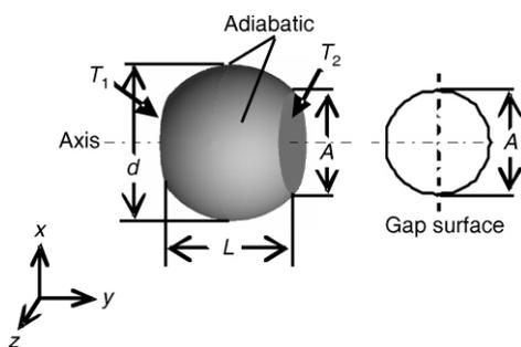
Figure 1. Geometry and boundary condition of spherical segment structure
