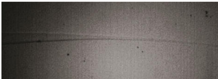
Figure 7. The shape variation of a stable jet observed in the optical microscope
