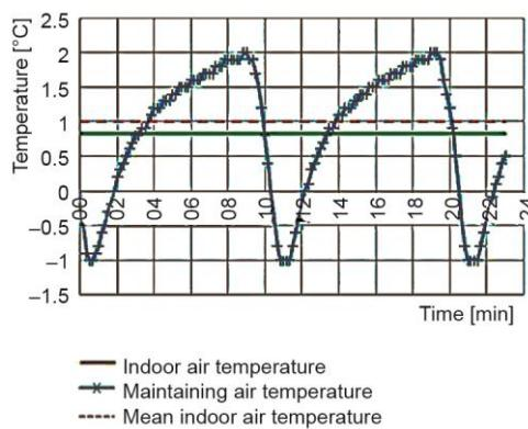
**Figure 5. Cabinet temperature at 1 °C maintaining air temperature with on/off controlled refrigerator**
