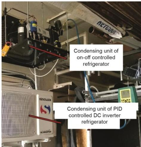
**Figure 1. Set-up of the condenser side of the test facility****Table 2. Specifications of on/off controlled condensing unit**
