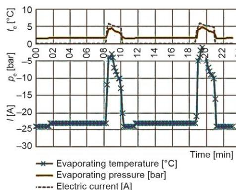
**Figure 6. Measured parameters at 1 °C maintaining air temperature with on/off controlled refrigerator**
