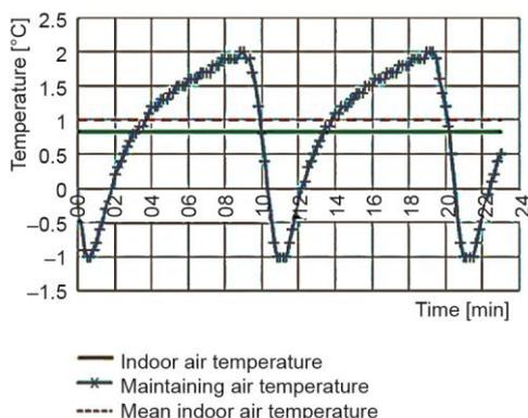
**Figure 5. Cabinet temperature at 1 °C maintaining air temperature with on/off controlled refrigerator**
