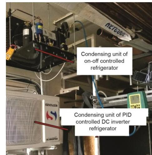
**Figure 1. Set-up of the condenser side of the test facility**
