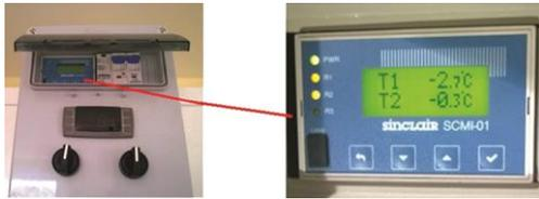
**Figure 4.** The PID control unit of the DC inverter refrigerator
