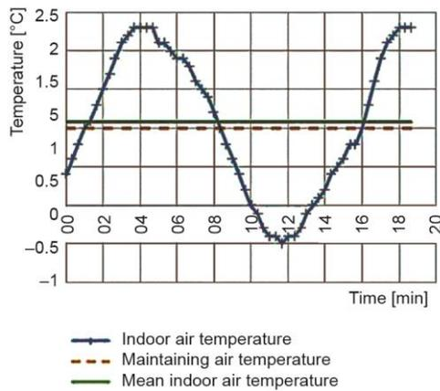
**Figure 7. Cabinet temperature at 1 °C maintaining air temperature with PID controlled refrigerator**
