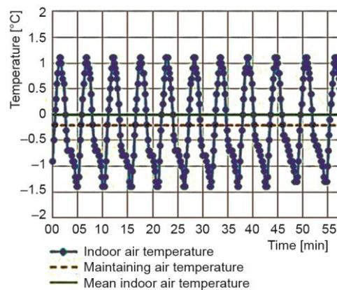
**Figure 9. Measured parameters at 0 °C maintaining air temperature with 500 W heat load with on/off controlled refrigerator**
