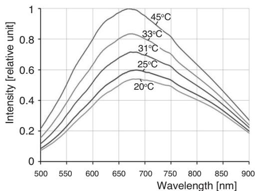
**Figure 2.** Changes in the relative intensity of light transmission vs. wavelength in the agarose gel with a 0.8% mass concentration
