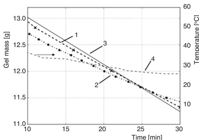
**Figure 4. Dependency of gel mass and temperature on time during liquid evaporation from gel surface:** (1) mass concentration of agarose 0.6%, (2) mass concentration of agarose 1.0%, (3) computations, (4) temperature in the gel volume
