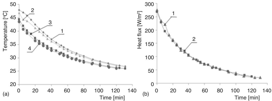
**Figure 5. Dependence of the temperature inside gel (a) and the heat flux for the outside wall of the experimental cuvette (b) on time during the gel formation: (1), (3) – mass concentration of agarose 0.6% (2), (4) mass concentration of agarose – 1.0%. On fig (a) the temperature is measured (1), (2) – in the center of the experimental cuvette filled with gel, (3), (4) – close to the inner wall**
