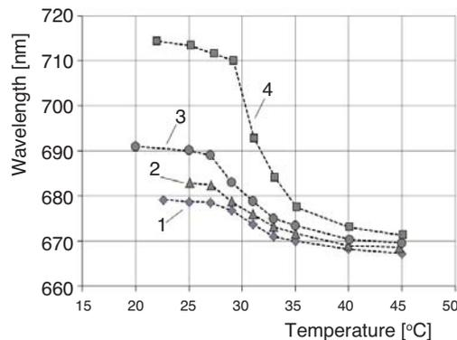
**Figure 3.** The change in maximum wavelength of the transmitted light, depending on the temperature of agarose gels formation and concentration; (1) 0.6%, (2) 0.8%, (3) 1.0%, and (4) 1.5%
