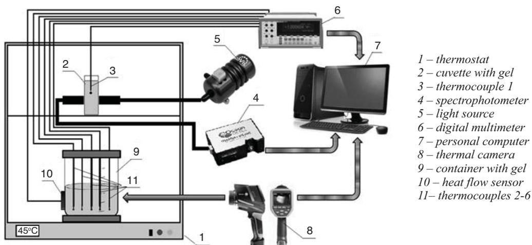
Figure 1. Scheme of the experimental set-up
