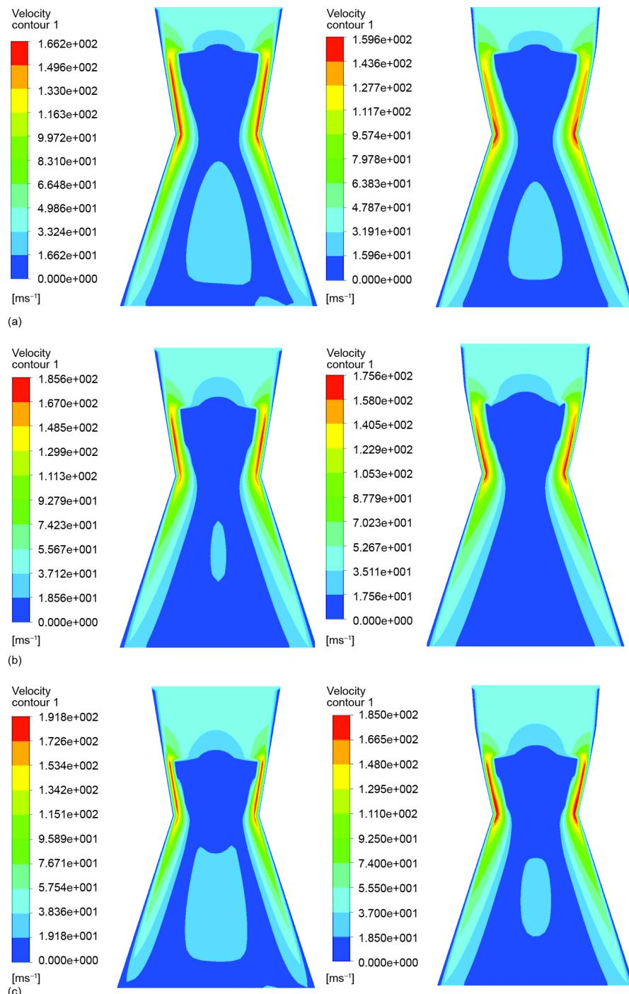
**Figure 3. Comparison of velocity distributions of conventional (left) and optimized (right) venturi scrubber designs for mound distances of (a) 0.1 m, (b) 0.4 m, and (c) 0.7 m**
