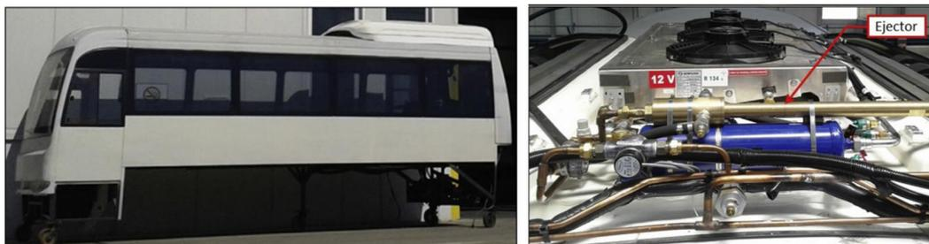
Figure 3. Ejector refrigeration system for bus
