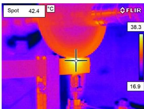
**Figure 5. Temperature distribution of downsized model of wheel-rail contact**
