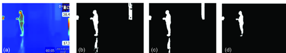
Figure 4. (a) thermal image, (b) segmentation results with manually determined threshold, (c) fuzzy segmentation results, (d) genetic algorithm optimized threshold (for color image see journal web-site)
