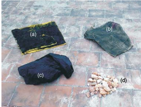
Figure 1(b). Photographic view of the wicks and pebbles used in the still; (a) black paint coated sponges, (b) black paint coated jute cloth, (c) black cotton cloth, and (d) pebbles
