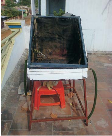
Figure 1(a). Photographic view of a SBSS with jute cloth (non-working model without glass cover)
