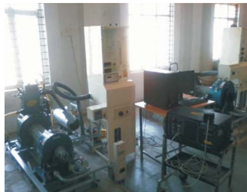
Figure 3. Pictorial view of engine test set-up
