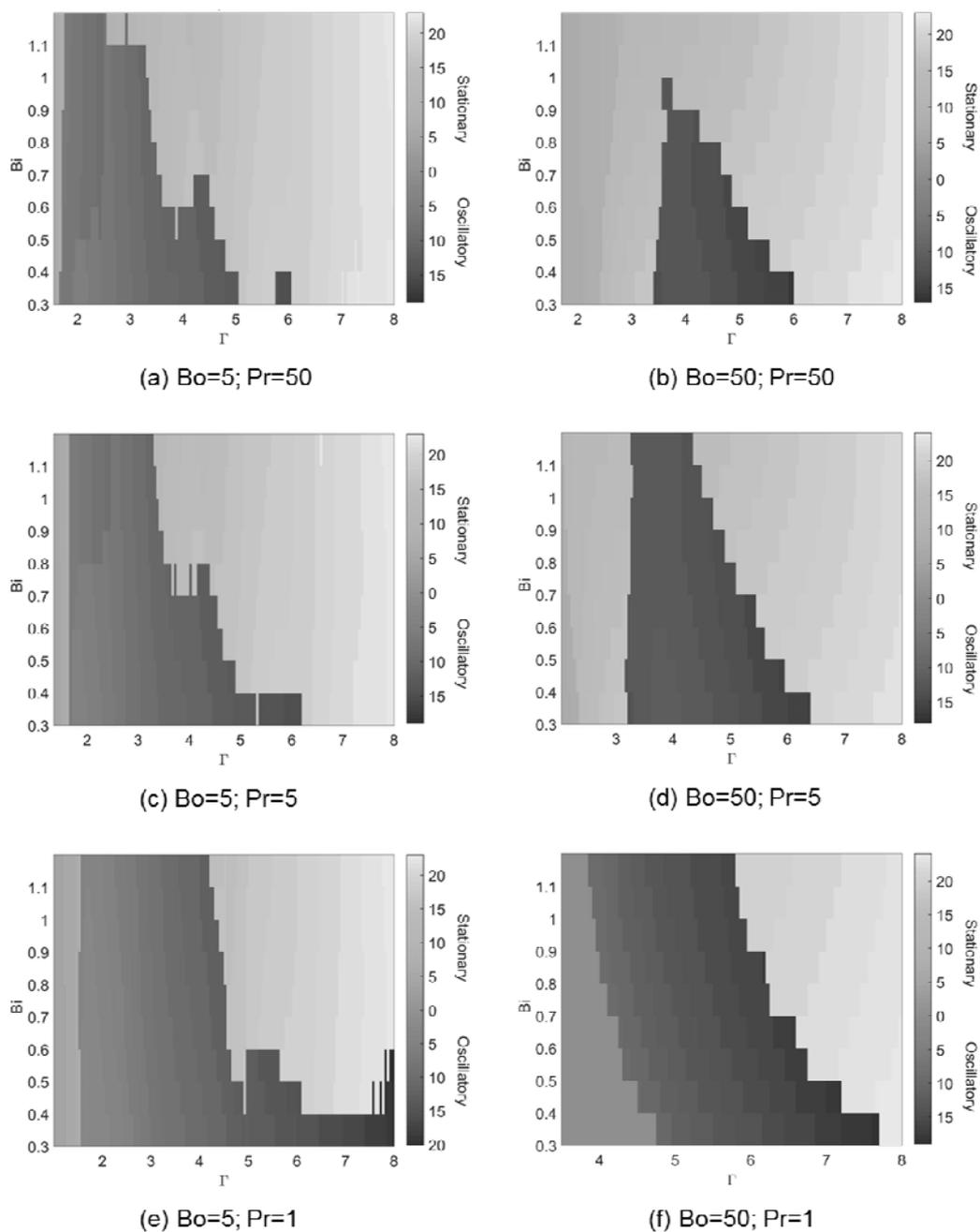
**Figure 2.** Critical wave number for the different numerical experiments analyzed in this work; the results are divided in stationary,  $\text{Imag}(\lambda) = 0$ , and oscillatory cases,  $\text{Imag}(\lambda) \neq 0$ ; left column cases with  $\text{Bo} = 5$  and for decreasing values of the Prandtl number and right column cases with  $\text{Bo} = 50$  (for color image see journal website)
