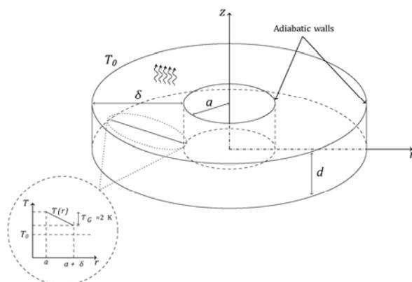
**Figure 1. Sketch of the domain. Lateral walls are considered adiabatic; the fluid is heated from below and the top surface is open to the atmosphere**
