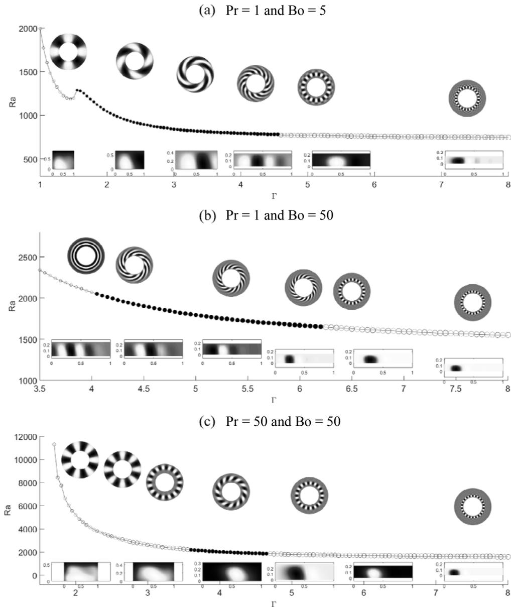
**Figure 3.** Evolution of the critical  $Ra$  with  $\Gamma$  for  $Bi = 0.8$ , and (a)  $Pr = 1$  and  $Bo = 5$ , (b)  $Pr = 1$  and  $Bo = 50$ , (c)  $Pr = 50$  and  $Bo = 50$ . Empty circles stand for stationary bifurcations, whereas bold ones indicate oscillatory ones; the size of the circle indicates the wave number in a scale from  $k = 0$  (the smallest circle) to  $k = 24$  (the largest one) (for color image see journal website)
