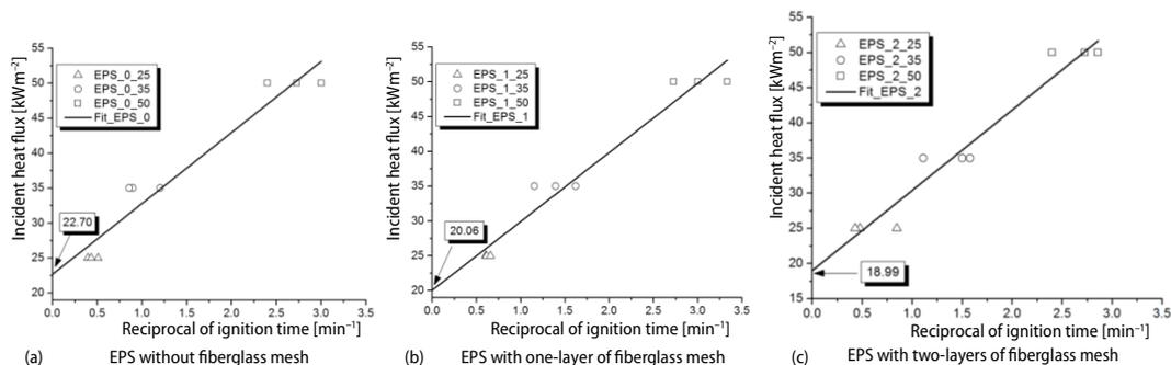
**Figure 3. Determination of the minimum heat flux required for ignition of EPS specimens**
