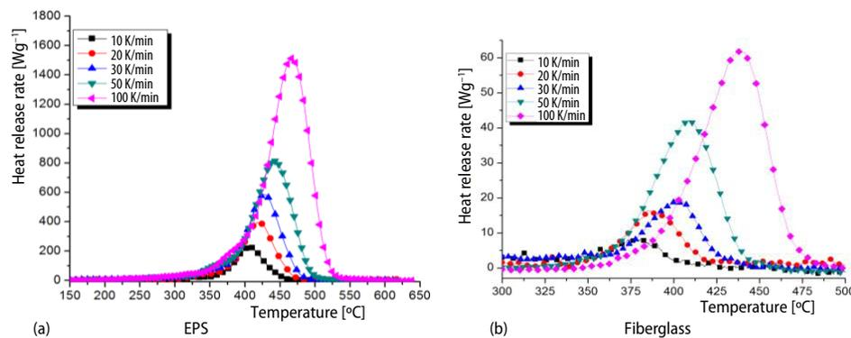
**Figure 2. The MCC heat release rate temperature curves**
