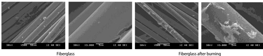
Figure 12. The SEM photos of fiberglass
