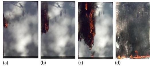
Figure 11. Burning of EPS with fiberglass
