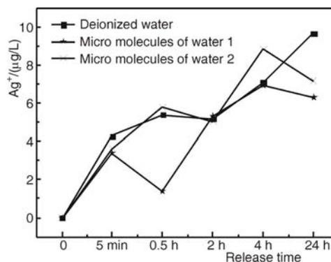
Figure 3. The relationship of the release concentration with the release time of the silver ions
