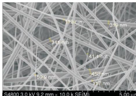
Figure 2. The SEM of nanofiber membranes
