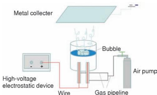
Figure 1. The device schematic diagram of bubble electrospinning
