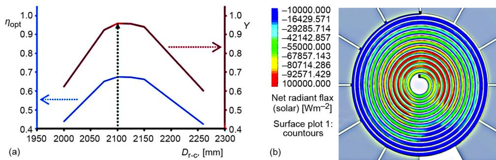
**Figure 2. Optical analysis of the collector; (a) optimization of the coil-reflector distance, (b) heat flux distribution of absorbed solar energy in the absorber down part**
