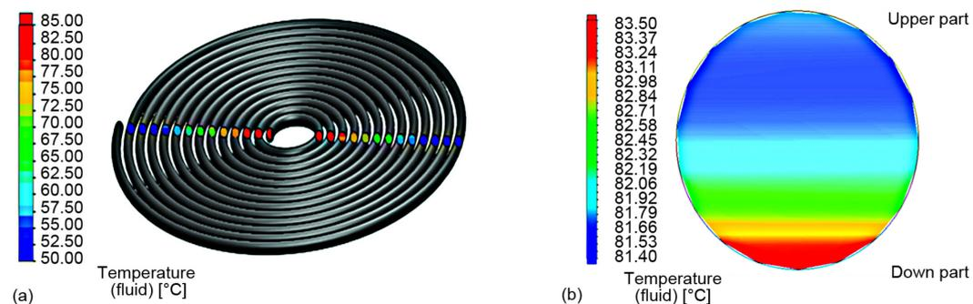
**Figure 6. Water temperature distribution; (a) in cross sections of the spiral coil, (b) distribution in the cross section of the outlet; the upper part of the figure presents the hotter down part of the coil**
