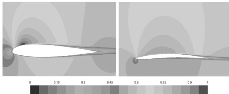
Figure 7. Mach number contours around the NACA 23015 and optimized airfoil using  $k-\varepsilon$
