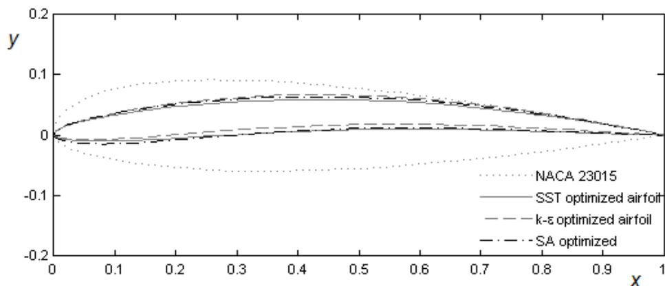
Figure 5. Airfoil shapes optimized with turbulence models in comparison with the NACA 23015
