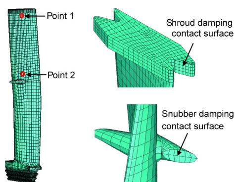
**Figure 1. The FEM model of a long steam turbine blade with snubber and shroud**
