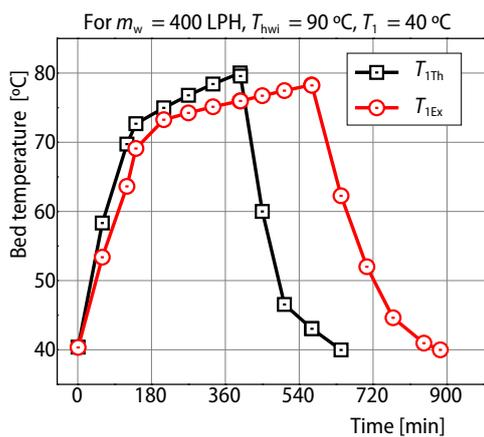
Figure 7. Variation of bed temperature during theoretical and experimental cycle (at  $T_1 = 40\text{ °C}$ )
