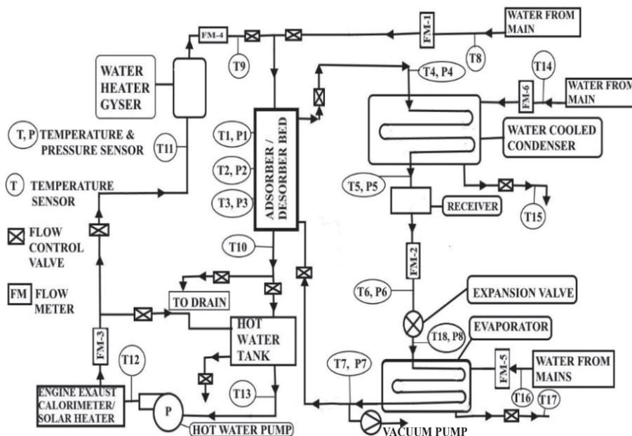
Figure 1. Schematic diagram [5] of the adsorption refrigeration system
