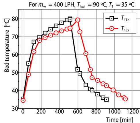
Figure 6. Variation of Variation of bed temperature during theoretical and experimental cycle (at  $T_1 = 35\text{ °C}$ )
