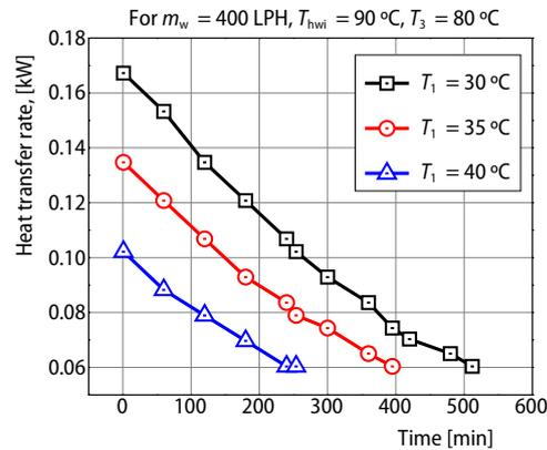
Figure 9. Variation of heat transfer rate to the bed with time during process 2 – 3
