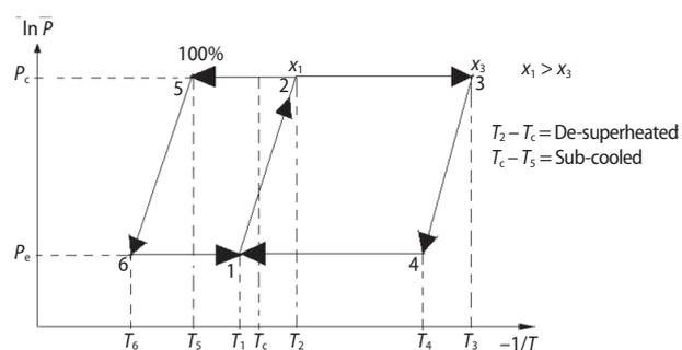
**Figure 2. The P-T-X diagram for a basic adsorption system [5]**
