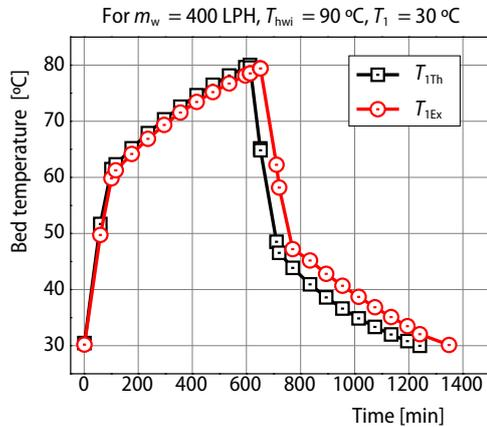
Figure 5. Variation of bed temperature during theoretical and experimental cycle (at  $T_1 = 30\text{ °C}$ )
