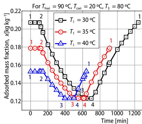
Figure 4. Variation of adsorption rate of refrigerant during simulated cycle
