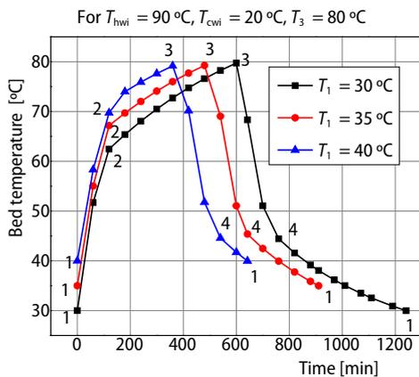
**Figure 3.** Variation of bed temperature during one complete cycle
