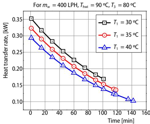
Figure 8. Variation of heat transfer rate to the bed with time during process 1-2
