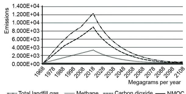
**Figure 5. Total emission of landfill gas, methane, CO<sub>2</sub>, and NMOC from the *Bubanj* landfill**
