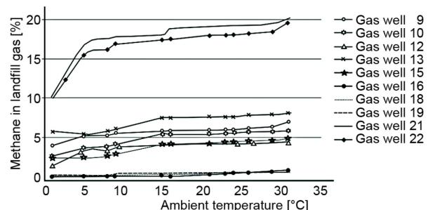
**Figure 7. Impact of ambient temperature on methane emission in section S4 of the *Bubanj* landfill**
