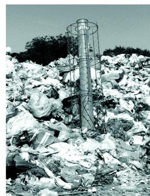
Figure 4. Measuring landfill gas emissions in the active section S4 of the Bubanj landfill
