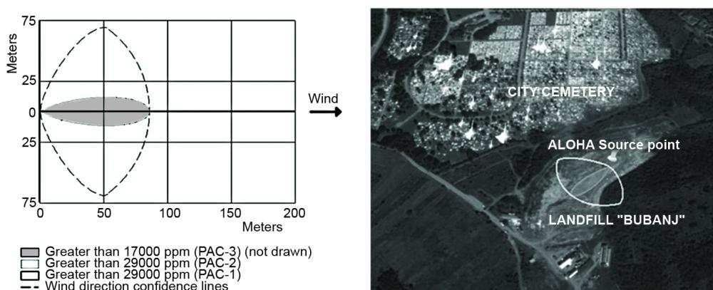
**Figure 8. Toxic zone caused by sudden emission of 100 kg of methane in section S4**
