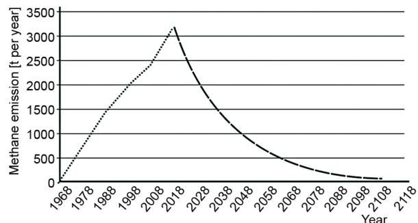
**Figure 6. Methane emission from the *Bubanj* landfill**
