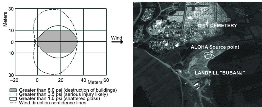
**Figure 10. Vulnerable zone after the ignition of 100 kg of methane in section S4**
