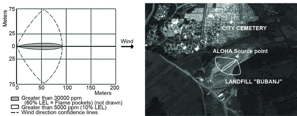
**Figure 9. Fire risk zone due to sudden emission of 100 kg of methane in section S4**
