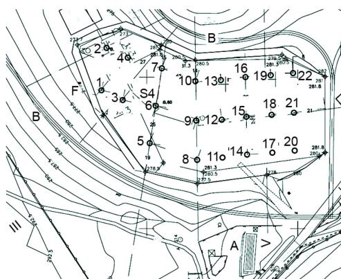
Figure 3. Layout of gas wells in the active section S4 of the Bubanj landfill
