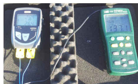
Figure 4. The actual photo of the solar meter and data logger that were used in this study
