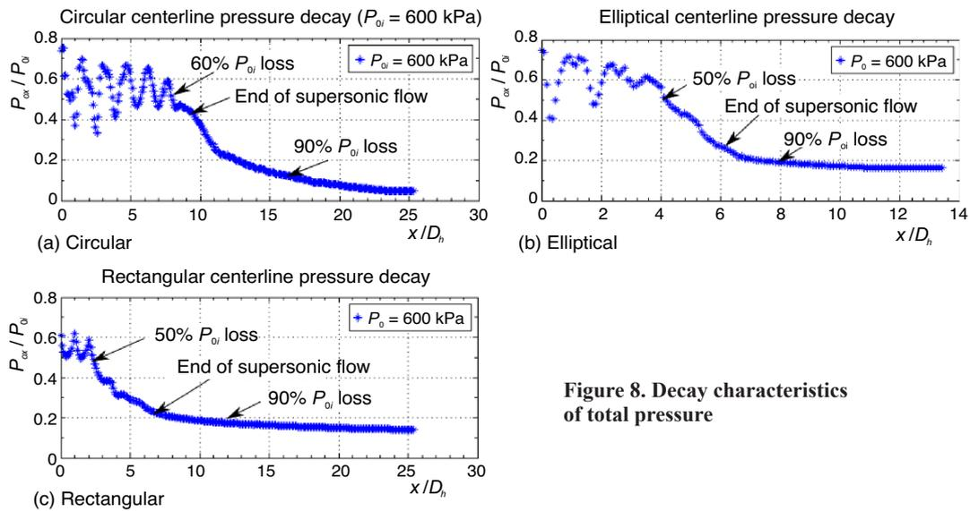
Figure 8. Decay characteristics of total pressure
