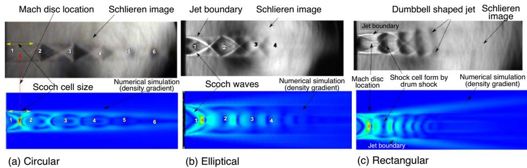
Figure 9. Schlieren image (major dimension) comparison with numerical simulation
