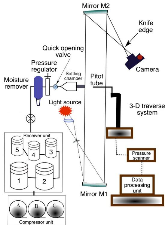
Figure 2. Experimental set-up
