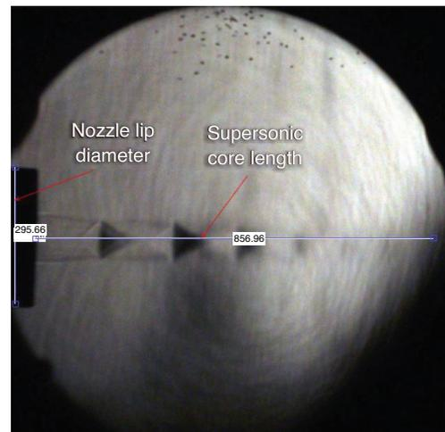
Figure 6. Typical Schlieren image
