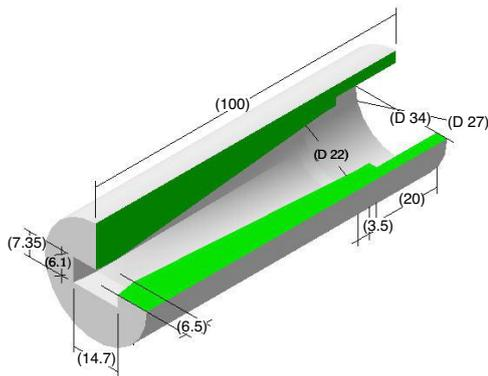
Figure 4 . Rectangular nozzle cut section
