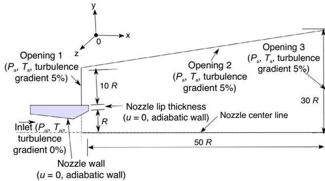
Figure 7. Computational domain and boundary conditions
