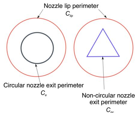
Figure 5. Typical exit geometry influencing parameters on decay characteristics
