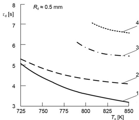
Figure 5. Ignition delay times of OCWF droplets depending on the oxidizer temperature during soaring in the combustion chamber
