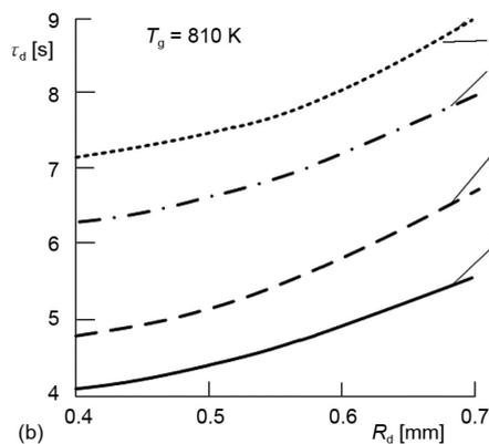
Figure 7. Ignition delay times of OCWF on the low-inertia thermocouple junction (type S, temperature measurement range is 273-1873 K, systematic error is  $\pm 1$  K, inertia is not more than 1 second, diameter of junction is about 0.1 second) depending on  $T_g$  (a) and  $R_d$  (b)
