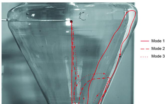
**Figure 4.** Videogram of experiment with a OCWF droplet (1<sup>st</sup> composition), when it soared in the combustion chamber during ignition (after post-processing in Tema Automotive) for conditions  $R_d \approx 0.5$  mm,  $T_g \approx 840$  K, and  $V_g \approx 1.5$  m/s
