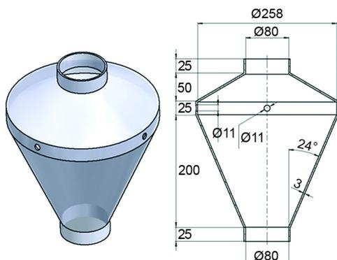
**Figure 2.** Developed combustion chamber made of quartz heat resistant glass (internal dimensions in mm)
