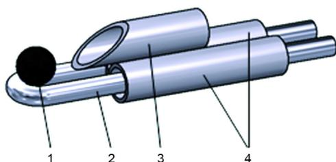
**Figure 3.** Scheme of dropping an OCWF droplet in the combustion chamber
