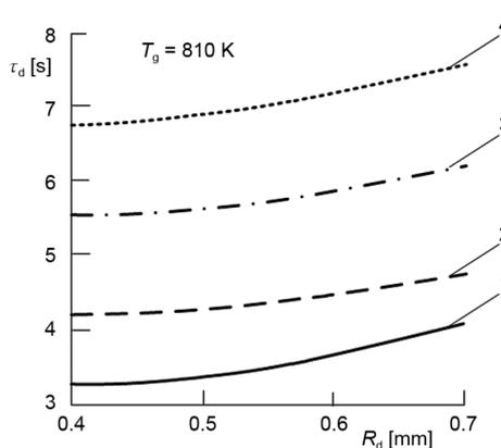
Figure 6. Ignition delay times of OCWF droplets depending on their size during soaring in the combustion chamber
