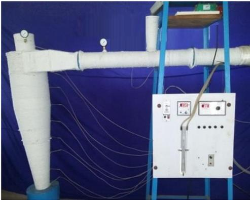
**Figure 9. Experimental set-up of cyclone heat exchanger**
