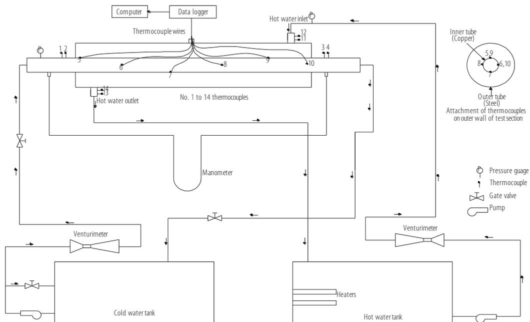
**Figure 3. Details of experimental set-up**
