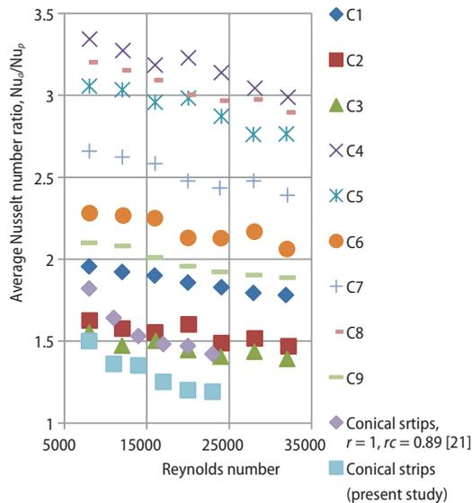
Figure 6. Average Nu ratio ( $Nu_a/Nu_p$ ) vs. Re
