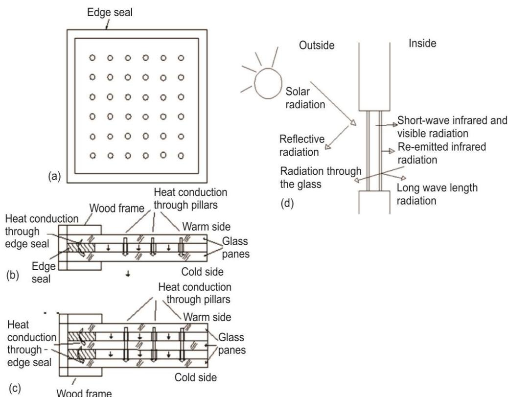
**Figure 1. Types of vacuum glazed windows and working principle; (a) plan view of double/triple vacuum glazing, (b) schematic of heat-flow through the double vacuum glazing, (c) schematic of heat-flow through the triple vacuum glazing [10-12], and (d) working principle of reduction in heat loss due to radiation**
