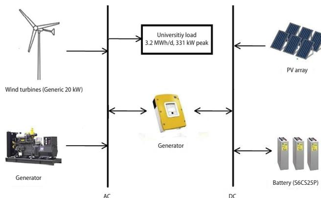
**Figure 5. Schematic diagram of the flow chart of energy**
