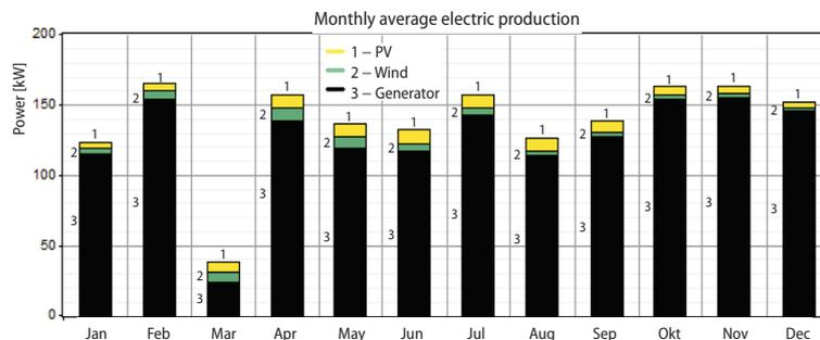
**Figure 8. Average monthly electric produced by diesel generator systems, PV and wind turbines separately during a year**
