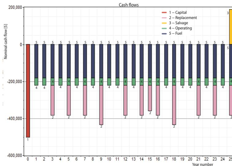
**Figure 6. Nominal cash flow (\$) during lifetime of the wind/diesel/battery hybrid system**
