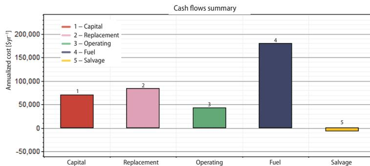
**Figure 7. Yearly cash flow summary for PV/diesel/battery hybrid system**
