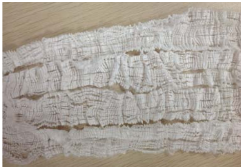
Figure 5. Crimped fibers by stuffer box crimping
