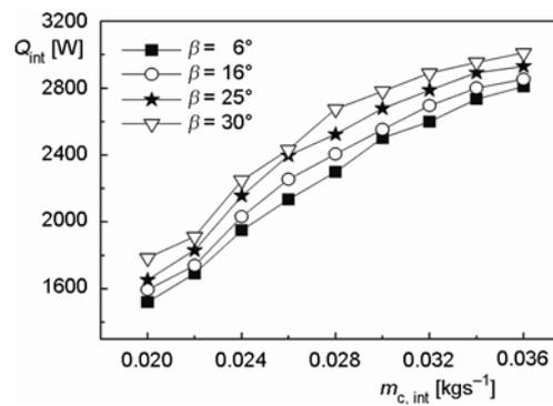
Figure 6. Variation of  $Q_{int}$  with  $m_{c,int}$ , under different spiral angle
