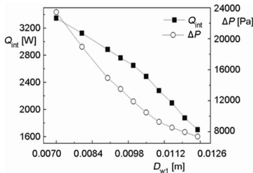
Figure 3. Variation of  $Q_{int}$ , and  $\Delta P$  with  $D_{w1}$
