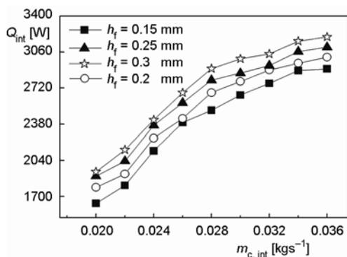
Figure 5. Variation of  $Q_{int}$  with  $m_{c,int}$ , under different  $h_f$
