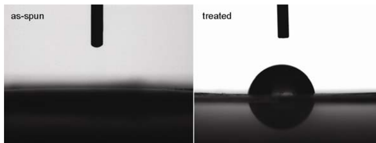
Figure 3. The WCA of as-spun and treated PVA nanofiber mat
