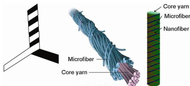
**Figure 1. Schematic diagram of fascinated nanofiber yarn in hierarchical structure**
