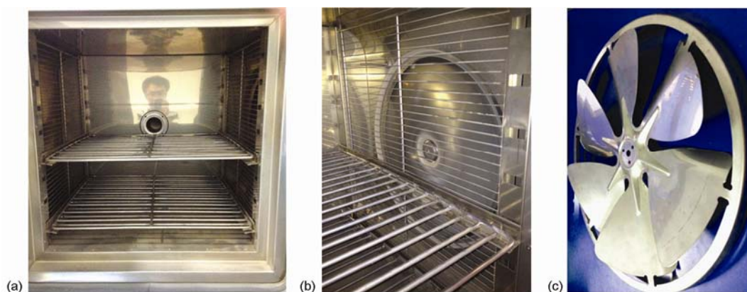
Figure 1. The physical model of the cigarette oven and impeller; (a) oven front view, (b) oven side face, (c) oven impeller
