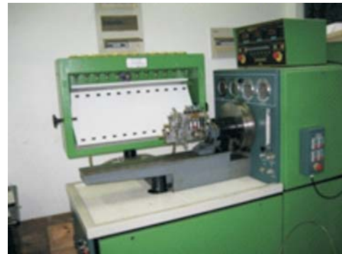
Figure 5. Oil pump test bench
