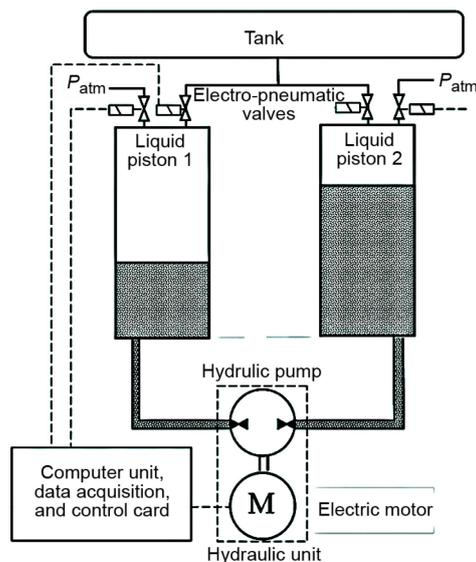
**Figure 1. Components of a small scale CAES system with liquid pistons**
