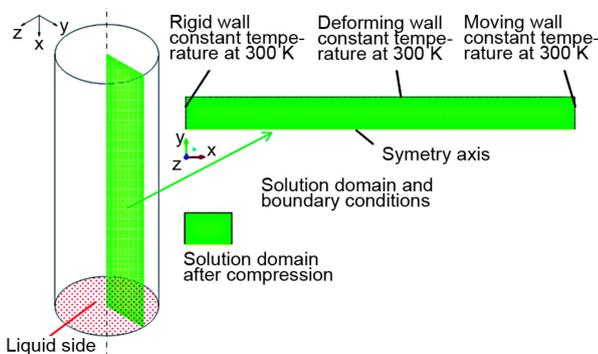
**Figure 2. Solution domain and the boundary conditions of the model**
