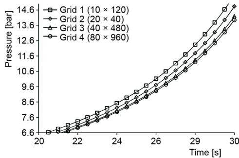
**Figure 3. Pressure values of different mesh sizes during compression**
