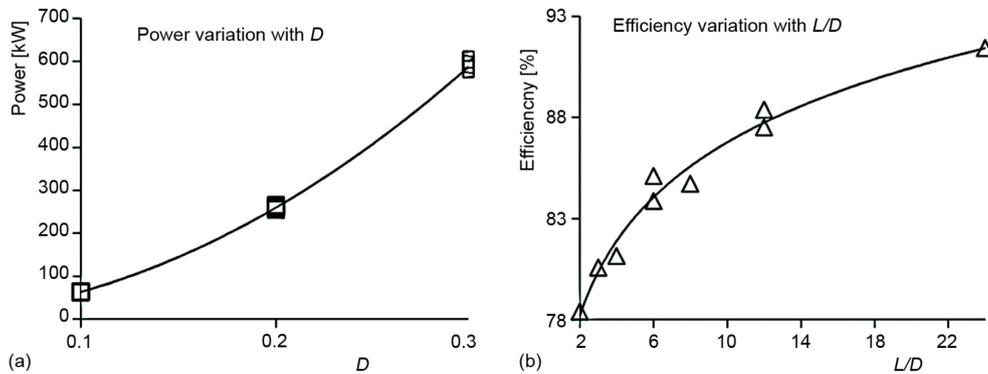
Figure 9. Power and efficiency variation with geometric parameters
