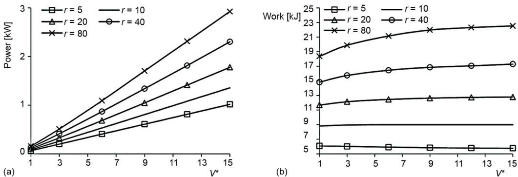
**Figure 8. Power and piston work variation with  $V^*$**
