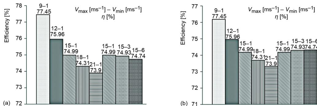
Figure 6. System efficiencies for variable piston speeds that calculated by the linear function (a) and quartic function (b)
