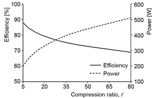
**Figure 7. Efficiency and power variation with compression ratio**
