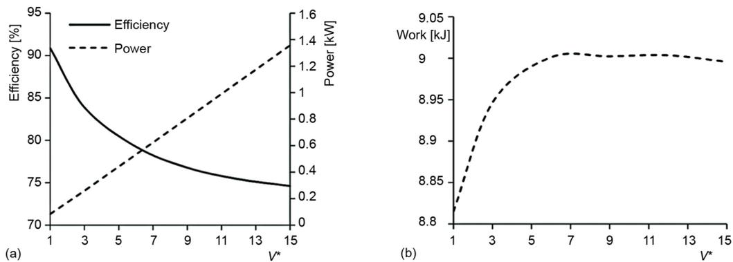
Figure 5. Variation of energy efficiency, power (a) and piston work (b) with non-dimensioned speed
