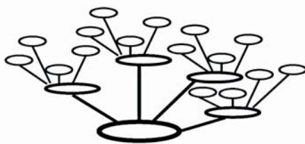
Figure 2. Schematic diagram of the hierarchic continuous tortuous channel path in the multilayer fabric
