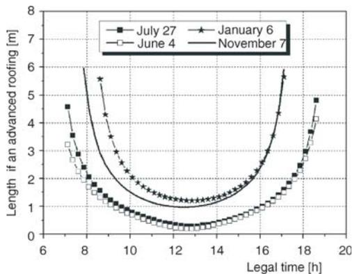
**Figure 5. Length variation of the advanced roofing**
