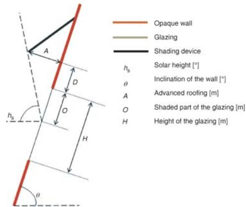
Figure 4. Integration of shading device
