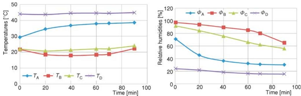
Figure 6. Drying air temperatures and relative humidities in the dryer depend on time
