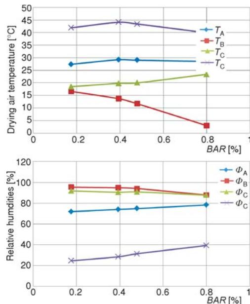
Figure 3. Changes in drying air temperatures and relative humidities depend on *BAR*
