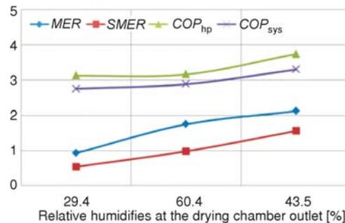
Figure 7. Changes of system parameter's depend on the relative humidity changes at the drying chamber outlet
