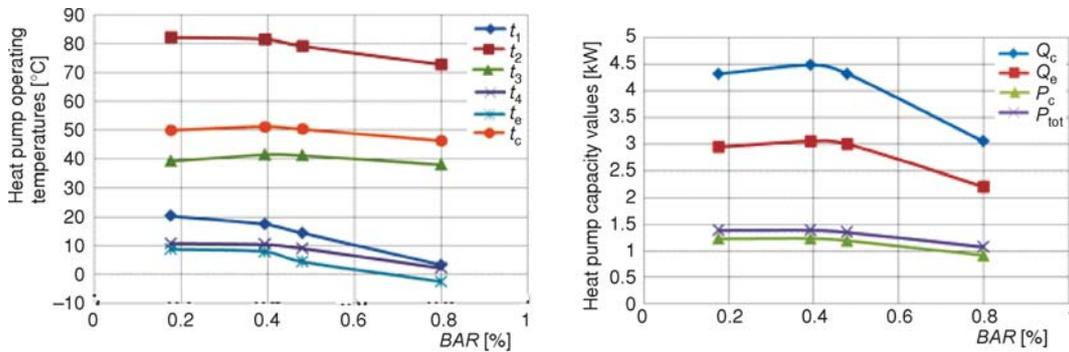
Figure 4. Changes in heat pump operating temperatures and capacities depend on  $BAR$
