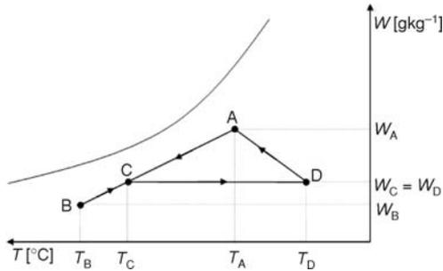
**Figure 2.** Change of the air properties during the drying process on the psychrometric diagram
